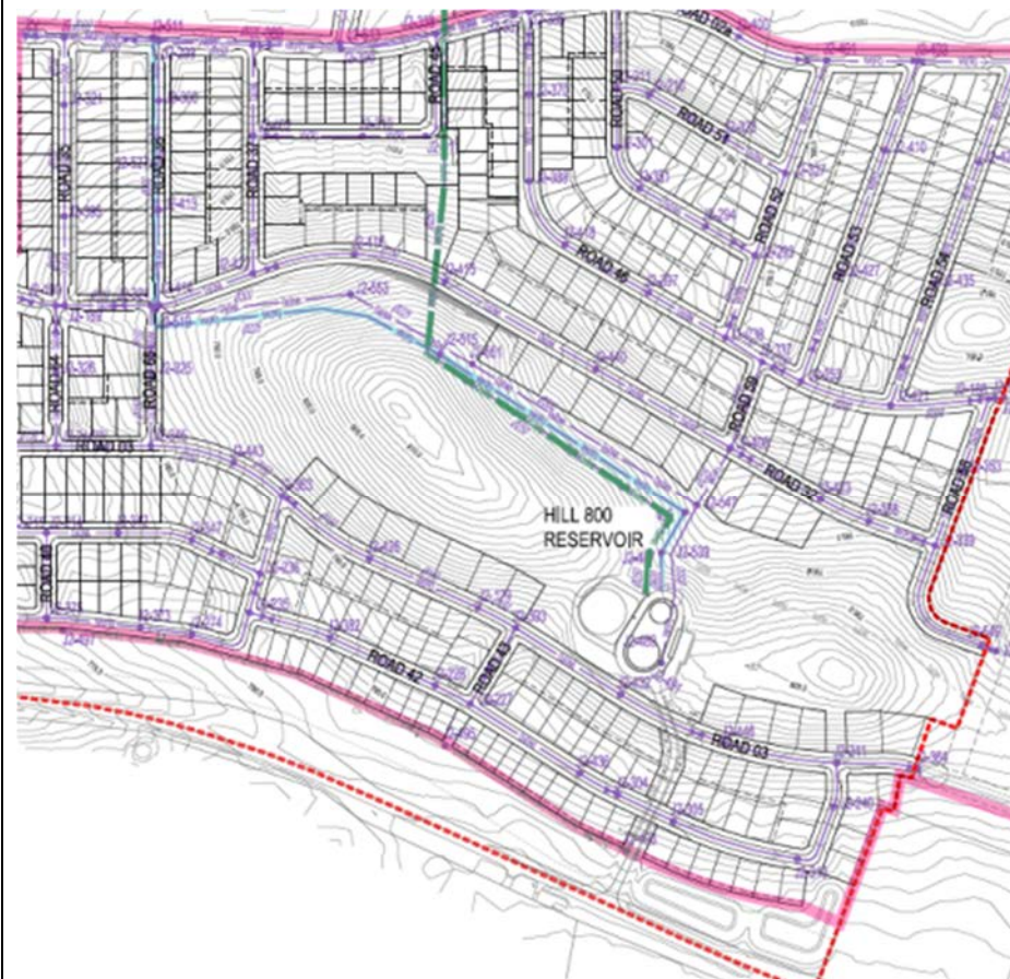
Figure 20: Hill 800 Recycled reservoir and water main distribution
